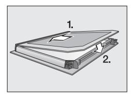
■ Push the inner pane into the plastic strip and insert it in the retainers.
